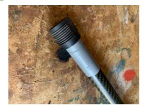
☐ Using a Hacksaw blade gently cut through the Nylon Clamp taking care not to cut the Carbon fibre shaft. Take your time doing this; you do not need to cut all the way through as the remaining plastic will crack when removing the clamp with pliers.
