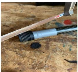
☐ Using pliers gently twist the plastic clamp and if cut through far enough will simply crack and come off the carbon shaft [There is no glue on the shaft]. If you can't crack the clamp simply cut a little deeper.
