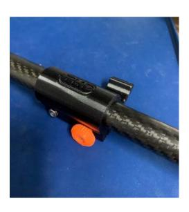
To maintain the clamps' life and effectiveness, ensure the detector shafts are kept free of dust when closing the detector.
