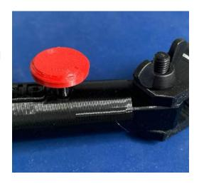
☐ When the pin has been fully pushed in the insertion tool can be removed and kept for later use.
