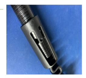
☐ Push the new swing arm hinge onto the shaft and align the holes to allow for the insertion of the locking pin. Hint: Push and turn the shaft slowly to align the holes.
